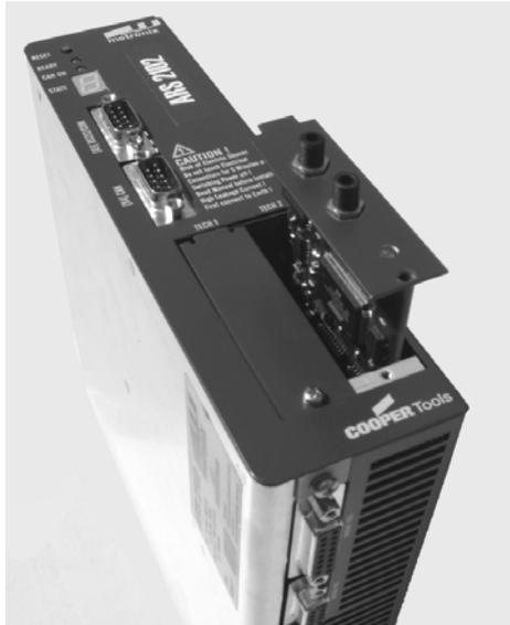
Figure 3.2: Plug-in position for ARS 2102, 2105, 2302, 2305 and 2310
