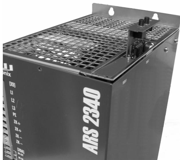
Figure 3.3: Plug-in position for ARS 2320 and 2340 and 2360W
